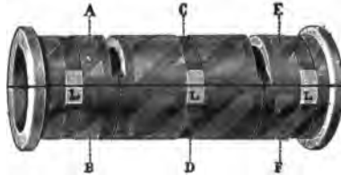
FIG. 144.—SLEEVE OF BABBITT METAL IN JOURNAL BEARING.
